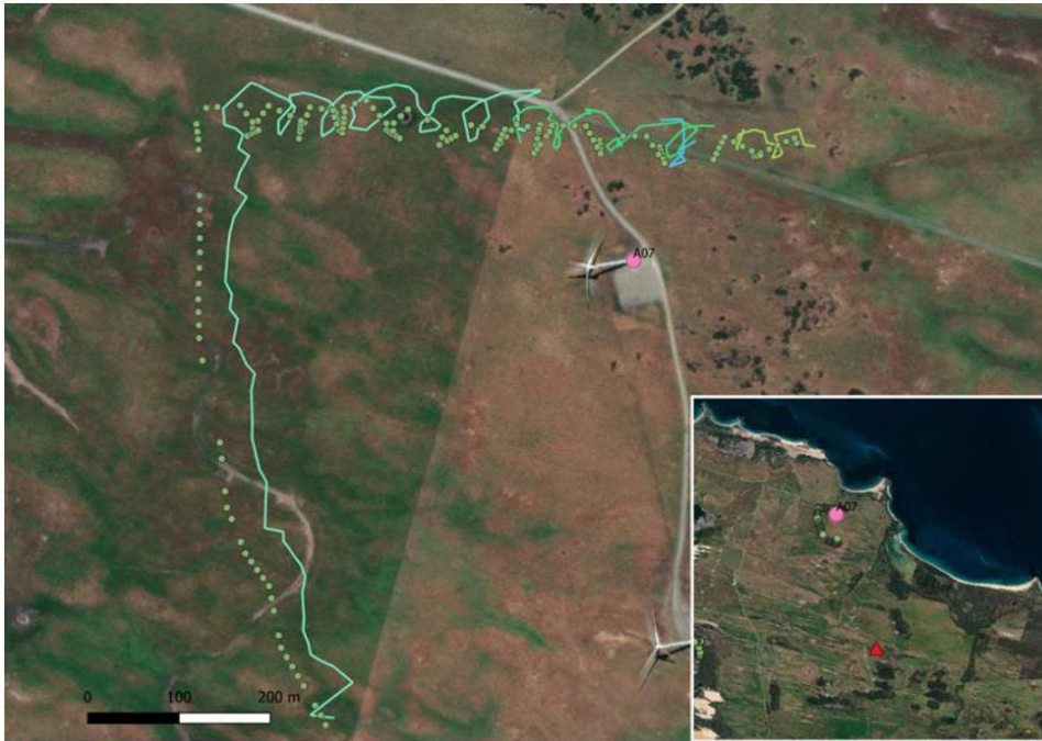
Figure 9. GPS track shown in dotted lines, compared with a broken radar track shown in solid lines (three separate tracks).
